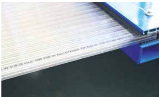
The ink-jet marks the UV-protected side of the sheet.
